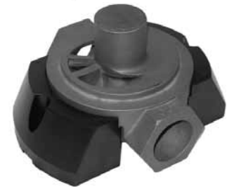
Valve body casting in 2 Jaw Power chuck
